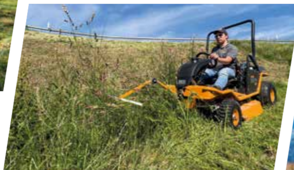
Insect-friendly Mowing with insect scare device
